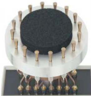
Figure 5: On the LHS, Uniform Circular Array (UCA) with N = 16 conical sensors (TU-Ilmenau). On the RHS, Uniform Rectangular Polarimetric Array (URPA) with N = 16 patch elements (HUT).
