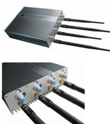
Figure: Typical generic quadband downlink jammer, probably about 10 W/band, probably made in China, probably jams a lot more than GSM.
