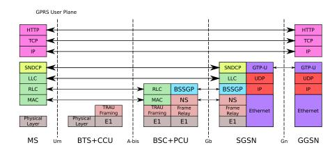
Circuit Switched Data (CSD) GPRS Stacking and Layers Core Network Protocols
