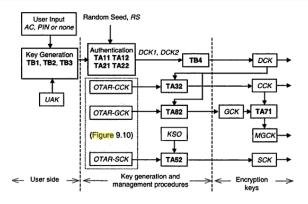
OTAR-CCK CCK sealed with DCK and received over the air interface
