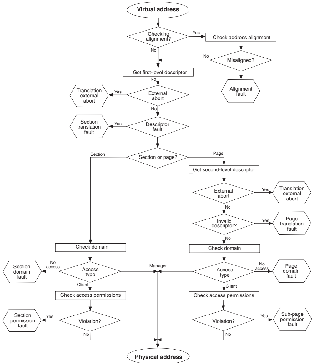
Figure 3-9 Sequence for checking faults
